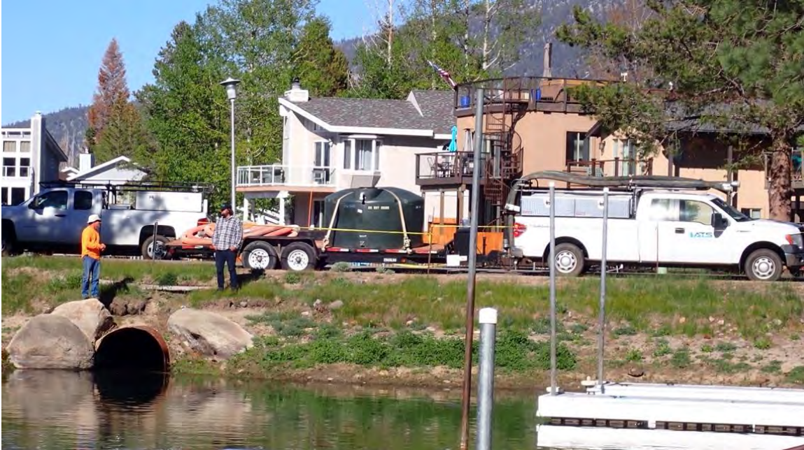
Figure 2-2. Example of Spill Prevention and Contingency Pumping Equipment Deployed During Herbicide Applications
