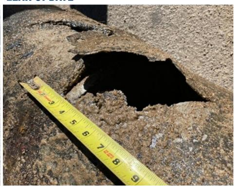
On February 8, 2022, the IVGID Effluent Pipeline experienced a leak causing damage to the roadway. This pipeline transports the treated sewage from Incline Village and Crystal Bay outside of the Lake Tahoe basin to the Carson Valley. Approximately 10,000 gallons of effluent water drained into a catch basin and snow. The District used a vacuum truck to remove all of the effluent remaining in the catch basin. No effluent flowed into Lake Tahoe.
