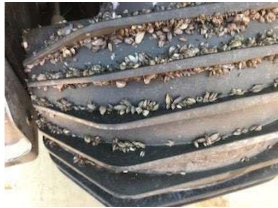
On July 18, the reverse bucket of the personal watercraft was found to have attached adult quagga mussels.
