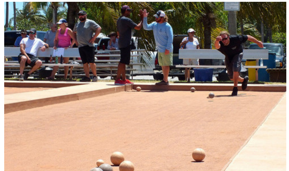
Bocce surfacing is typically a loose surface material such as decomposed granite. Crushed oyster shell or a specialty bocce mix is the preferred surface for many players. Maintenance and removal of leaves and debris should be considered during site design.
