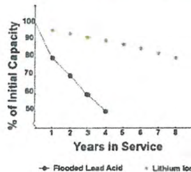
Battery Capacity Years in Service
