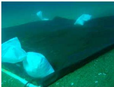
10-foot by 10-foot rubber bottom barriers were tested as a strategy for managing Asian clam populations
