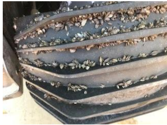
The reverse bucket of the personal watercraft was found to have attached adult quagga mussels.
