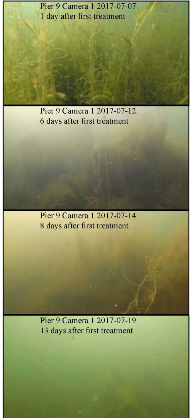
Photo 4. Photo documentation over a 16-day period following UV-C light treatment in the LSM, June 30, 2017 through July 19, 2017
