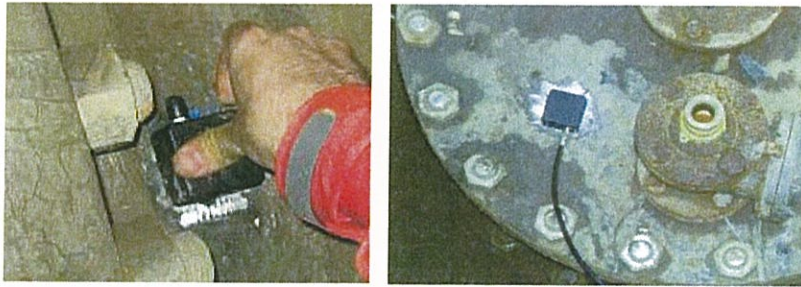
Figure 2: Example SMS Acoustic Sensor Glued to Flange
