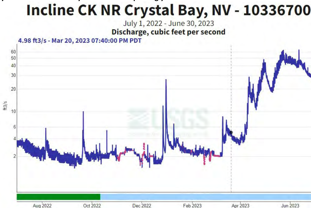
Figure 1.3: Incline Creek surface water discharge in cubic feet per second from July 1, 2022- June 30, 2023, provided by the USGS gauge 10336700 2 . March 20, 2023, is highlighted as the filtration avoidant purveyor maximum turbidity date for the reporting year.
