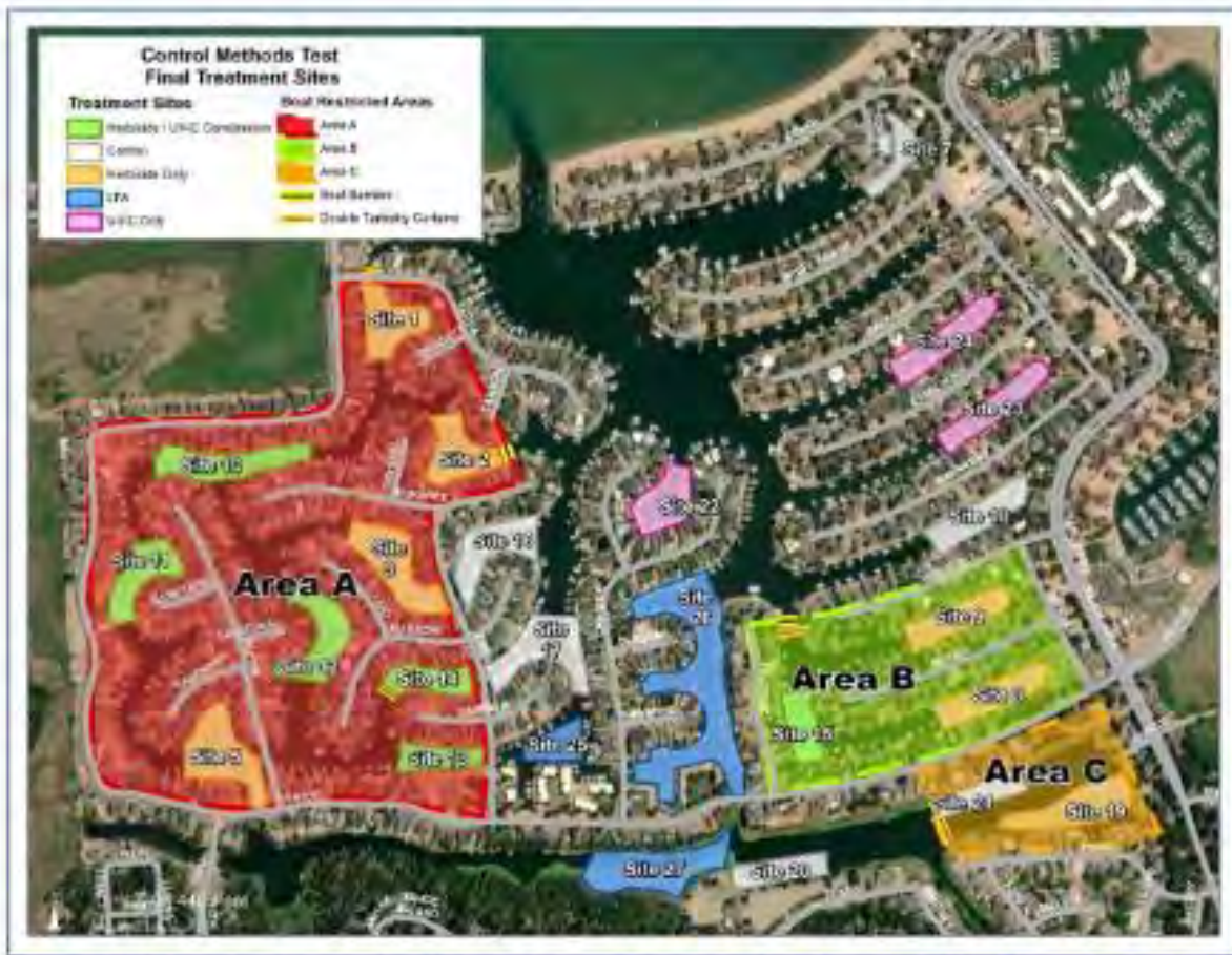
Figure 3. Map depicting restricted boating areas separated from the West Lagoons by sets of double turbidity curtains (A, B, and C) and boat barriers (A and B). The shaded zones also show where boating entrance and egress was prohibited from pre-herbicide applications (May 25, 2022) until removal of barrier curtains from each area.
