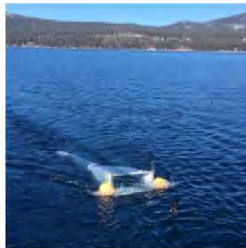
Manta trawl skims the water, collecting microplastics from Lake Tahoe's surface. Photo: K. Senft
