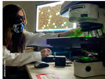
Research Associate Jackelyn Lang analyzes microplastic samples with Raman microspectroscopy in the Gjeltema lab.
