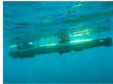
Autonomous Underwater Vehicle (AUV) is used to map clam beds around Lake Tahoe
