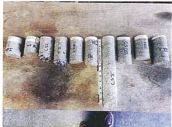
Pool Photo #10 Core samples for testing. Note, two from wading pool, two from pool deck and six from swimming pool.
