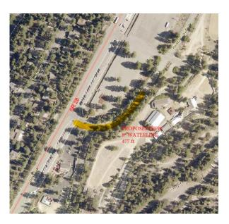
Based on information from Pipeline Staff, Engineering has identified this waterline as one to be replaced as part of a future CIP Waterline Replacement project; however, this particular project is still a few years out in budget planning.
