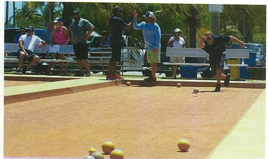
Bocce surfacing is typically a loose surface material such as decomposed granite. Crushed oyster shell or a specialty bocce mix is the preferred surface for many players. Maintenance and removal of leaves and debris should be considered during site design.
