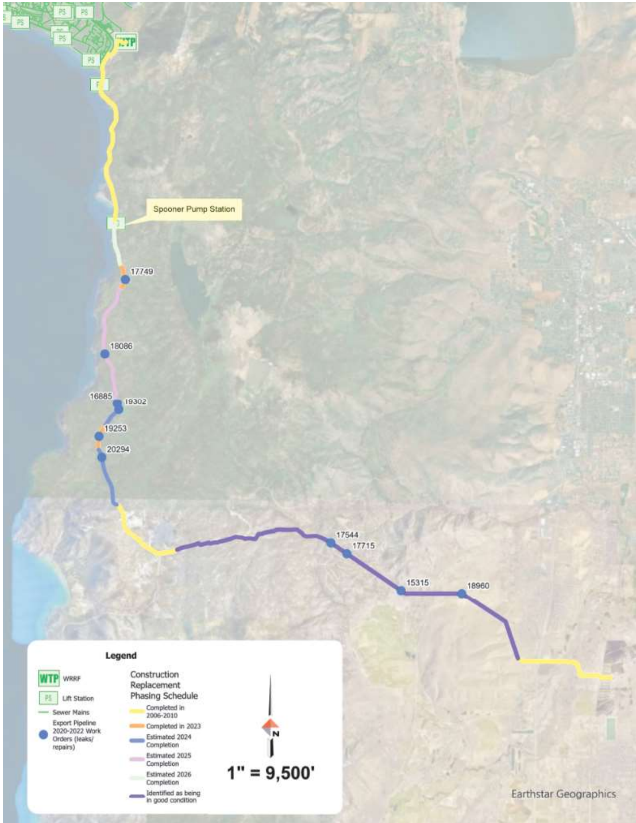
Figure 87: Export Pipeline Leaks /Issues (2020-2022)
