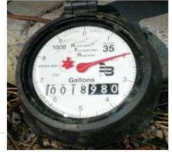
Water Meter Register
